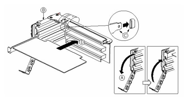
Figure 23: Installing a PCI card of the riser
